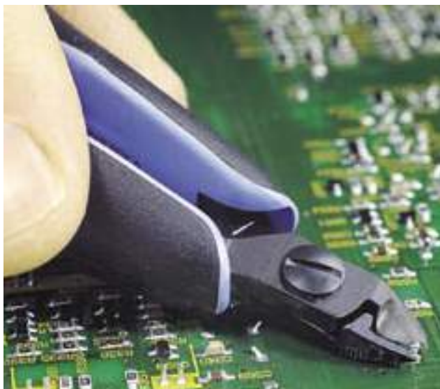
The Rx8140 used in traditional over-hand grip. See page 40 for more on Rx8140.
