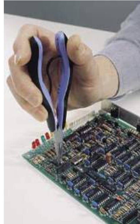
The Rx7890 in an inverted grip is used to straighten a connector pin. See page 46 for more on Rx7890.
